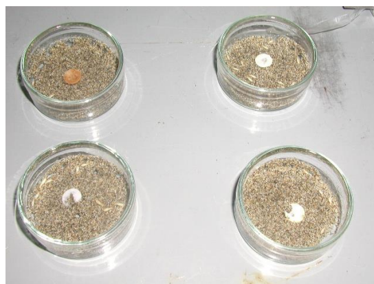
Figure 2. No-choice test against Reticulitermes speratus termites using paper discs.
