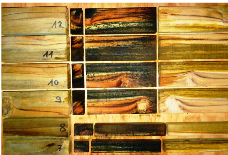
Figure 2. CCA treated test specimen from Australia. (Source: Norton 2012).
