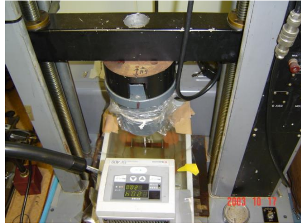
Figure 1. Static bending tests in a water bath.
