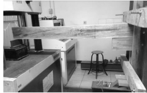
Figure 7. Testing process of the Meranti Timber Beam-Column Joint Connection.
