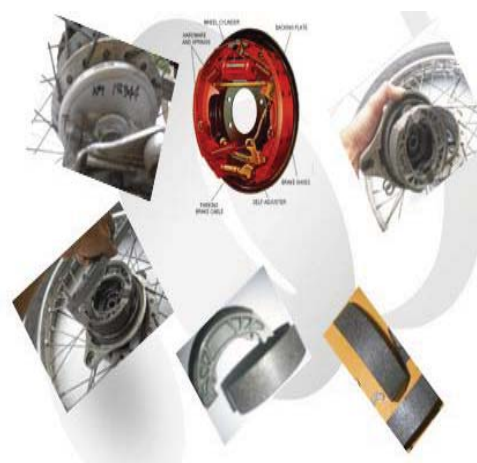
Figure 3. Specimen of pulp fiber brake lining testing, brake shoe type (Source: howstuffworks.com & Wawan KH and Posma RP).
