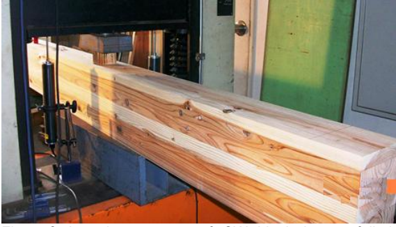
Figure 3. Insertion process of CW block into a full-size beam.
